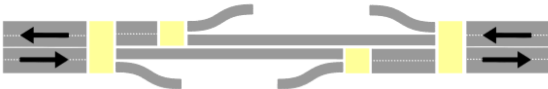
Figure: scheme of an entry / exit situation. The yellow rectangles represent simple junctions that connect the incoming and outgoing roads. Each gray line represents a separate road, the leftmost and rightmost roads contain lanes of both driving directions.
